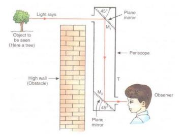
The figure shows a tree behind a high wall which we cannot see directly. We can, however, see this tree by using a periscope as follows:
