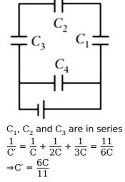
All the capacitors in branch 1 is in series so the charge on each capacitor is  $Q' = \frac{6}{11}CV$ Also charge on capacitor  $C_4$  is Q = 4CV $\therefore$  Ratio  $= \frac{Q'}{Q} = \frac{6CV}{11 \times 4CV} = \frac{3}{22}$
