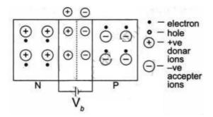
This results from the concentration of immobile charges close to the junction after electrons and holes diffuse across the function.
