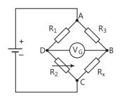
The resistance is adjusted until the bridge is 'balanced' and no current flows through the galvanometer. At this point, the voltage between the two mid-points (B and D) will be zero.
