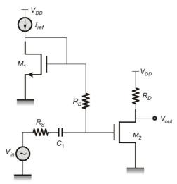
Assuming that capacitor  $C_1$  is a short circuit for AC analysis, the exact magnitude of small signal voltage gain  $\left| \frac{V_{Out}}{V_{in}} \right|$  is \_\_\_\_\_.
