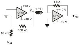
Assume that the initial inductor current is 0 A. The input voltage ( $V_i$ ) is a triangular signal with peak voltages of  $\pm 2$  V and time period of 8  $\mu$ s. Which one of the following statements is true?
