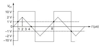
$V_{01}$  is square wave. It is delayed by 1  $\mu$ s wrt input  $V_i$ .
