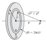
The electric potential of each ring, of radius r and width dr, have charge dq is given by  $\sigma \, dA = \sigma 2 \, \pi r dr$
