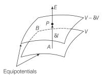
Here, the figure electric field is always remain in the direction in which the potential decreases steepest. Its magnitude is given by the change in the magnitude of potential per unit displacement normal to the equipotential surface at the point.
