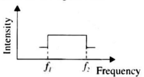
Assume that the sound of the whistle is composed of components varying in frequency from  $f_1 = 800 \text{ Hz}$  to  $f_2 = 1120 \text{ Hz}$ , as shown in the figure. The spread in the frequency (highest frequency – lowest frequency) is thus 320 Hz. The speed of sound in still air is 340 m/s.
