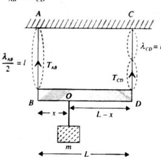
For rotational equilibrium of massless rod taking torque about point O,
