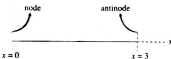
The fixed end is a node while the free end is an antinode. Therefore, at x = 0 is a node and at x = 3 m is an antinode. Possible modes of variation are
