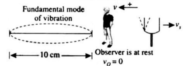
The frequency of tuning fork as heard by the observer standing stationary near sonometer wire can be found with the help of Doppler effect.
