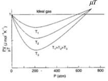
Experimentally value of  $\frac{PV}{\mu T}$  for real gas was calculated by altering the pressure of gas at different temperatures. The graphs obtained have been shown in the diagram. Here for the purpose of comparison, graph for an ideal gas has also been drawn, which is a straight line parallel to pressure axis.
