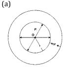
Let r =radius of a spherical liquid drop of Centre O, T = surface tension of the liquid. Let  $P_i$  and  $P_0$  be the value of pressure inside and outside the drop.
