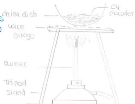
• oxidation of copper to CuO.
