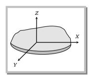
*Example*: Moment of inertia of a disc about an axis through its centre of mass and perpendicular to its plane is  $\frac{1}{2}MR^2$ , so if the disc is in x-y plan perpendicular axes
