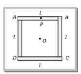
Solution: (a) Moment of inertia of rod AB about point  $P = \frac{1}{12}Ml^2$
