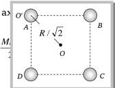
$I_O = I_{O'} + M \left(\frac{R}{\sqrt{2}}\right)^2 = \frac{2}{5}Mr^2 + \frac{MR^2}{2}$  [by the theorem of parallel ax Moment of inertia of system (i.e. four sphere) =  $4I_O = 4\left[\frac{2}{5}Mr^2 + \frac{M}{2}\right]$
