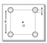
Solution: (b) M. I. of sphere A about its diameter  $I_{O'} = \frac{2}{5}Mr^2$
