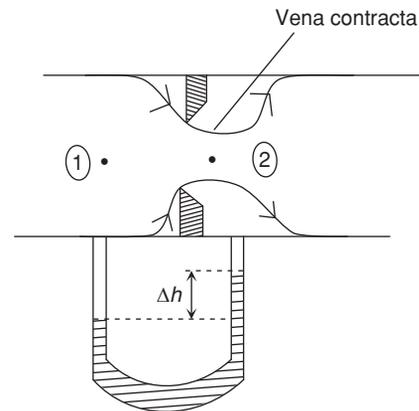
The flow through the orificemeter from an upstream section contracts until a section downstream, where the vena contracta is formed, and then expands to fill the whole pipe. One of the pressure tapings is usually provided at the upstream of the orifice plate where the flow is uniform and the other is provided at the vena contracta. At the vena contracta, streamlines converge to a minimum cross section.
