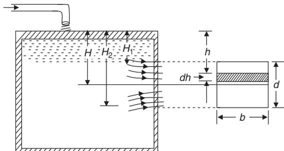
Consider a large rectangular orifice of with  $b$  and height  $d$ , fitted to one vertical side of a large tank, discharging freely into atmosphere, under a constant  $H$  as shown in figure.
