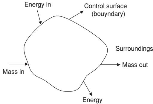
A control volume is an open system with a boundary called the control surface. Transfer of mass and energy takes place across the control surface. A deforming control volume has a changing volume while the volume of a non-deforming control volume is fixed.
