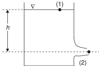
The flow is assumed to be incompressible and irrotational. The draining of the water is slow enough that the flow can be assumed to be steady (quasi-steady). Any losses in the nozzle are neglected. Point 1 is taken to be at the free surface of water and so  $p_1 = p_{\text{atm}}$  and point 2 is taken to be at the centre of the outlet area of the nozzle and so  $P_2 = P_{\text{atm}}$
