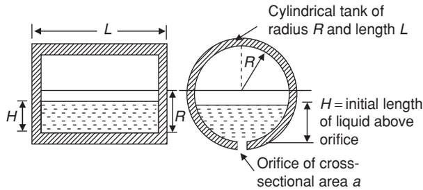
**Figure 5** Time for emptying a circular horizontal tank through an orifice at its bottom
