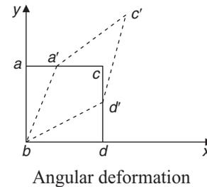
In a two-dimensional flow field in Cartesian coordinates, translation without deformation and rotation is possible if the velocity components  $u$  and  $v$  are neither a function of  $x$  nor of  $y$ . When a velocity component is a function of only one space coordinate along which that velocity component is defined, e.g.,  $u = u(x)$  and  $v = v(y)$ , then translation with linear deformation is possible.
