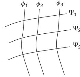
Flow nets are used to study 2-dimensional irrotational flow especially in cases where the stream and velocity functions are unavailable or difficult to solve.
