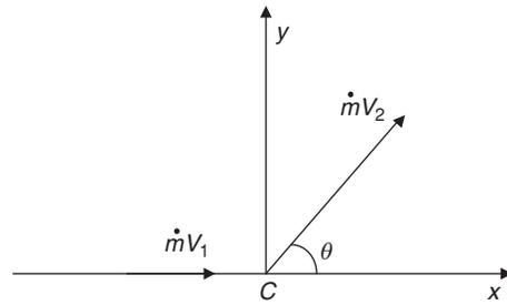
**Figure 2** Linear momentum of fluid at inlet and outlet
