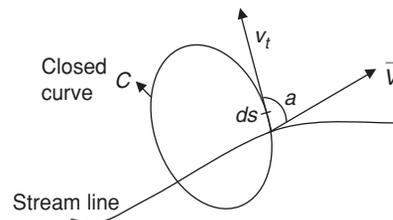
Circulation  $\Gamma$  is defined as the counterclockwise line integral, around a closed curve  $C$ , of arc length  $ds$  times the velocity component tangent to the curve ( $v_t$ ) in the flow field.
