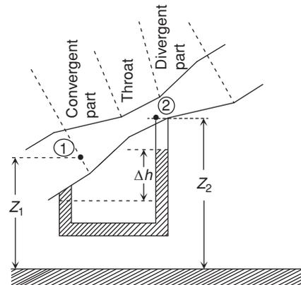
From the Bernoulli equation and the continuity equation, the velocity at the throat is obtained as follows.
