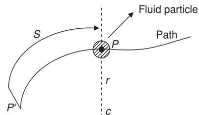
Let  $S$  denote the distance travelled by the particle along the path line relative to the reference point  $P'$ ,  $t$  denote time and  $v (=f(s, t))$  denote the speed of the particle. Let  $\hat{i}$  be a unit vector tangential to the path at point  $P$  and let  $\hat{n}$  be a unit vector normal to the path at point  $P$  and pointing inward towards the centre of curvature  $C$ . Let  $r$  denote the radius of curvature at point  $P$ .
