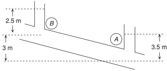
19. Water is pumped from a large tank as shown in the figure below. The head loss is known to be equal to  $\frac{6V^2}{2g}$ , where  $V$  is the discharge velocity, and the pump head is equal to  $20 - 5Q^2$ , where  $Q$  is the discharge. If the discharge pipe has a diameter 100 mm and if only SI units are considered, then the discharge  $Q$  is equal to:
