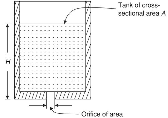
**Figure 3** Time for emptying a tank of uniform cross-sectional area through an orifice at its bottom
