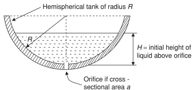
**Figure 4** Time for emptying a hemispherical tank through an orifice at the bottom
