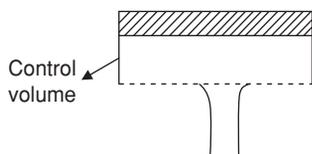
Applying the linear momentum balance equation for the control volume shown above, we get  $-250 = \dot{m}(0 - v_2)$  (momentum correction factor is assumed to be unity)
