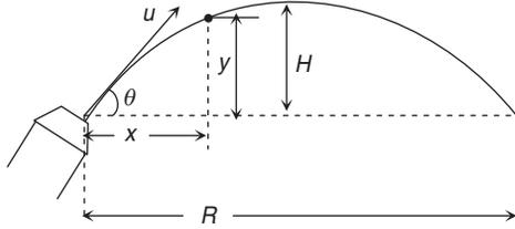
Here  $u$  is the velocity of the liquid jet and  $\theta$  is the angle made by the jet with the horizontal. The equation of the jet is:
