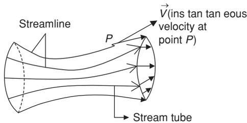
On steady flows, the shape and position of a stream tube does not change.
