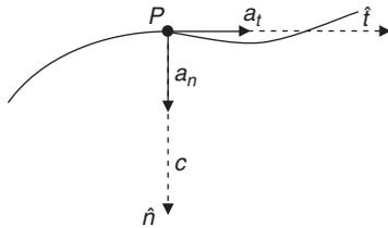
The *tangential component* of the acceleration vector,  $a_t = \left( v \frac{\partial v}{\partial s} + \frac{\partial v}{\partial t} \right)$  and the *normal component*,  $a_n = \frac{v^2}{r}$ .
