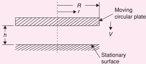
12. The radial velocity  $V_r$  at any radius  $r$ , when the gap width is  $h$ , is: [2008]
