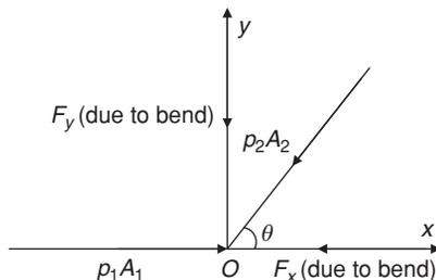
**Figure 1** Forces on fluid due to pressures and due to bend
