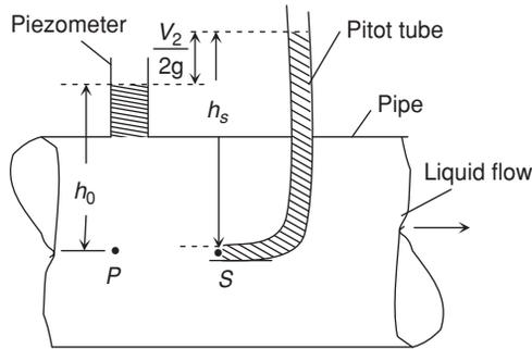
Point  $S$  is a stagnation point while point  $P$  is a point in the undisturbed flow both being at the same horizontal plane.
