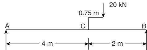
A simply supported beam  $AB$  is loaded at point  $C$  at a distance 4 m from  $A$ , as shown in figure. Flexural rigidity of the beam is 15,000 kN-m<sup>2</sup>. Deflection at point  $C$  is
