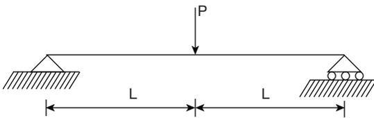
Strain energy stored in the beam with flexural rigidity  $EI$ , loaded as shown in the figure is
