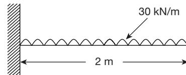
Maximum shear force is at the fixed end and is
