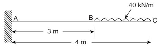
A cantilever is loaded as shown in the figure. If flexural rigidity is  $36 \times 10^4$  kN-m<sup>2</sup> deflection at point C is
