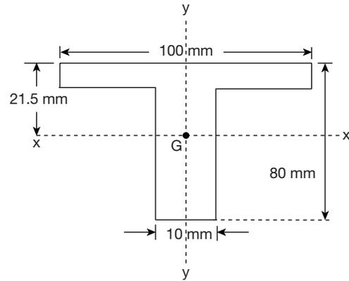
For a column of cross section as shown above and length 3 m has one end fixed and other end free. Values of Young's modulus and moments of inertia are as follows
