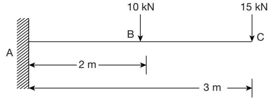
For the cantilever loaded as shown in figure, value of flexural rigidity is  $4 \times 10^4$  kN-m<sup>2</sup>. Deflection at the end C is
