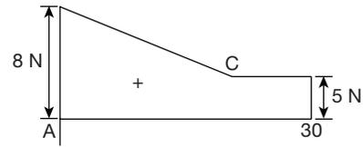
At point B the shear force is 5 N and is constant up to C and due to UDL the shear force increases linearly to 8 N at point A.
