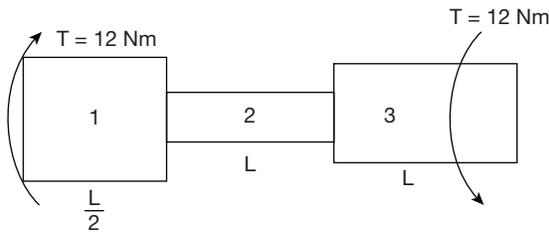
A shaft as shown in figure is subjected to a torque 12 Nm at the ends. Torsional stiffness of the portions 1, 2 and 3 of the shaft are 40 Nm/rad, 20 Nm/rad and 30 Nm/rad respectively. Angular deflections between the ends is
