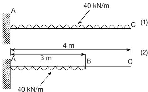
Loading of the beam can be split into as shown below
