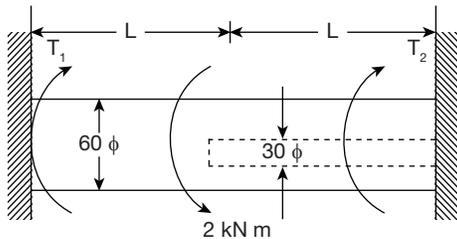
A shaft of length  $2\ell$  and outside diameter 60 mm fixed at both ends is subjected to a torque of 2 kN-m at the centre. Half of the shaft is hollow with inside diameter 30 mm. The ratio of reaction torques  $T_1$  and  $T_2$  at the ends is
