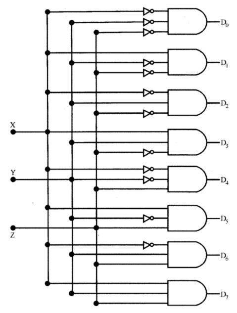
The circuit is designed with AND and NAND logic gates. It takes 3 binary inputs and activates one of the eight outputs. 3 to 8 line decoder circuit is also called as binary to an octal decoder.
