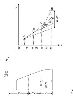
Let  $t_{B/A}$  be the vertical distance of point B from the tangent to the elastic curve at point A. This distance is termed as the tangential deviation of B with respect to A.
