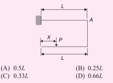
10. A frame is subjected to a load P as shown in the figure. The frame has a constant flexural rigidity EI. The effect of axial load is neglected. The deflection at point A due to the applied load P is [2014]
