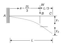
Deflection at  $B = \frac{Wa^3}{3EI} = y_1$ Since there is no load in the portion *BC*, Slope  $\left(\frac{dy}{dx}\right)_B$  is maintained throughout the portion slope at  $B = \frac{Wa^2}{2EI}$ Deflection at  $C = y_1 + y_2 = \frac{Wa^3}{3EI}, \quad \frac{Wa^2}{2EI} \times \frac{L}{3}$  $= \frac{Wa^2}{3EI} \left(a + \frac{L}{2}\right)$ putting  $a = \frac{2L}{3}, \quad C = \frac{14}{81} \frac{WL^3}{EI}$
