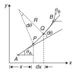
The figure shows elastic curve AB of an initially straight beam (exaggerated).
