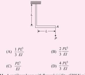
A cantilever beam with flexural rigidity of 200 N.m<sup>2</sup> is loaded as shown in the figure. The deflection (in mm) at the tip of the beam is \_\_\_\_\_. [2015]
