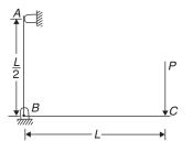
A frame *ABC* with 2 arms is hinged at *B* and loaded at free end *C* as shown in the figure. Each arm of the frame has a flexural rigidity *EI*.
