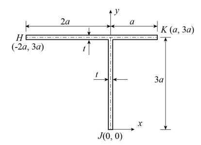
The coordinates of the shear center of this cross-section are:
