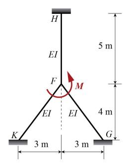
If the magnitude (absolute value) of the support moment at H is 10 kN-m, the magnitude (absolute value) of the applied moment M (in kN-m) to maintain static equilibrium is \_\_\_\_\_\_. (round off to the nearest integer)
