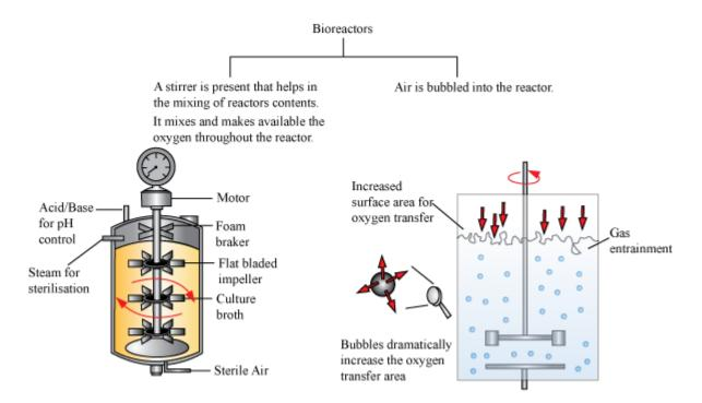
• A bioreactor has the following components - agitator system, oxygen delivery system, foam control system, temperature and pH control system, sampling ports.
