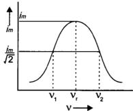
Phase difference ( $\phi$ ) in series LCR circuit is given by  $\tan \phi = \frac{X_C - X_L}{R}$ For resonant  $\phi = 0 \Rightarrow X_C - X_L = 0$
