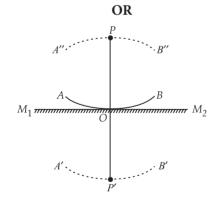
In figure, *P* is a point object placed at a distance *r* from a plane mirror  $M_1M_2$ . With *P* as centre and *PO* = *r* as radius, draw a spherical arc; AB. This is the spherical wavefront from the object, incident on  $M_1M_2$ .
