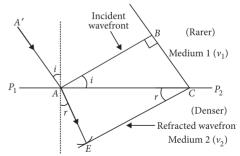
Let  $v_1$  and  $v_2$  represents the speed of light in medium 1 and medium 2 respectively. We assume a plane wavefront *AB* propagating in the direction *A'A* incident on the interface at an angle *i*. Let *t* be the time taken by the wavefront to travel the distance BC.
