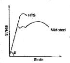
Both mild steel and HTS has nearly the same slope for the stress-strain curve, i.e., same Young's modulus.
