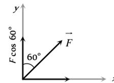
The component of force in vertical direction
