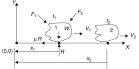
Change in kinetic energy from position 1 to 2 is  $(\Delta \text{ KE})_{1-2}$ =  $\frac{1}{2}m(v_2^2 - v_1^2)$
