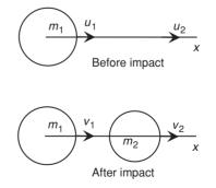
It is assumed that these velocities are directed along the line joining the centres of the two spheres and, are considered to be positive if they are in the positive direction of the *X*-axis. This is called the case of direct central impact. Two equal and opposite forces, i.e., action and reaction, are produced at the point of contact during impact. According to the law of conservation of momentum, such forces cannot change the momentum of the system of two balls, hence:
