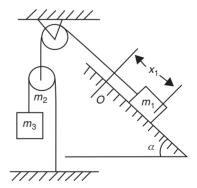
configuration can be completely specified by one coordinate, such as  $x_1$  in the above figure. In the case shown in the above figure, for example, the assumptions involve a smooth inclined plane, frictionless bearings, inextensible
