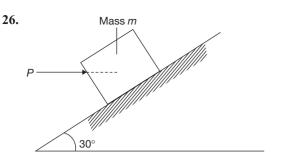
A block of mass m is in equilibrium on an inclined plane of 30° by the action of an horizontal force P as shown in the figure. The value of the force is
