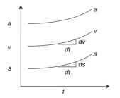
Considering the general case of acceleration not being a constant, the above graphical representation is made.
