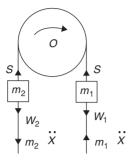
The inertia of the pulley and the friction on its axle are assumed to be negligible. If the motion of the system is assumed to be in the direction as shown by the arrow on the pulley, an upward acceleration  $\ddot{x}$  of the weight  $W_2$  and a downward acceleration  $\ddot{x}$  of the weight  $W_1$  is obtained. The inertia forces acting on the corresponding weights are shown in the above figure.
