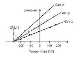
Graph of pressure versus temperature (in °C) at constant volume.
