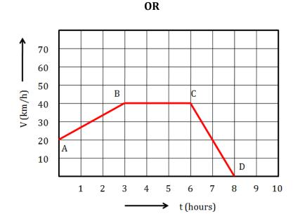
(a) Acceleration between points A and B will be given by the slope of line AB.
