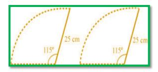
It can be observed from the figure that each blade of wiper will sweep an area of a sector of  $115^{\circ}$  in a circle of 25 cm radius.
