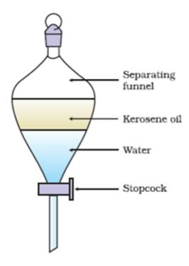
Kerosene Oil having low density settles to the top of water and water is easily obtained by opening the stopcock of the funnel.
