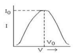
The variation of current with frequency of a.c. source in series LCR circuit
