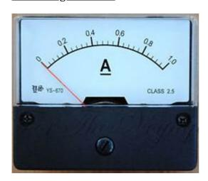
This is Ammeter used to measure current in the circuit. Electric current is measured in ampere (A) that is why letter capital A is written on the device scale.
