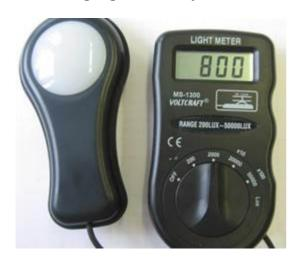
This is photometer generally used to measure the light intensity.
