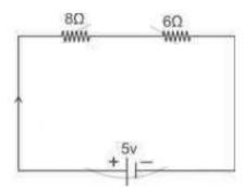
Calculate potential difference across the  $8\Omega$  resistor.
