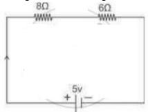
A third resistor is now connected in parallel with  $6\Omega$  resistor. Will the potential difference across the  $8\Omega$  resistor the larger, smaller, or the same as before? Explain the reason for your answer.
