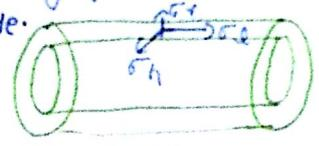
$\sigma_r$  in thickness  $\rightarrow$  Tensile
