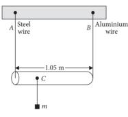
cross-sectional areas of wires A and B are  $1.0 \text{ mm}^2$  and  $2.0 \text{ mm}^2$  respectively. At what point along the rod should a mass m be suspended in order to produce (a) equal stresses and (b) equal strains in both steel and aluminium wires?
