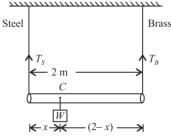
Let a weight W be suspended at a distance x from steel wire. Let  $T_S$  and  $T_B$  be tensions in the steel and brass wires respectively.
