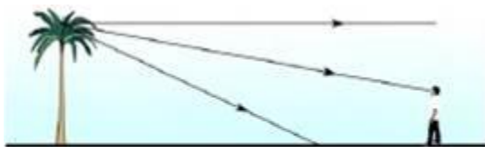
fig-9(b): The paths of light rays when there is no change in density of air
