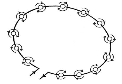
As shown if fig. each section of wire produces its concentric set of lines of force. By applying right hand thumb rule, we find that all the section produce magnetic field directed downward at all points inside the loop while at the outside points, the field is directed upwards. Hence the magnetic field acts normally into the place of paper at the points inside the loop and normally out of the plane of paper at points outside the loop.
