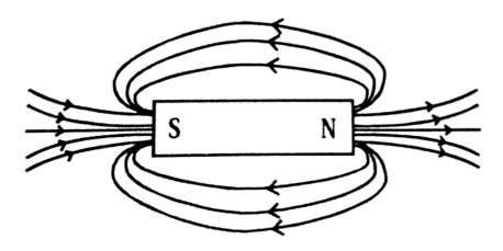
Fig : Field lines around a bar magnet
