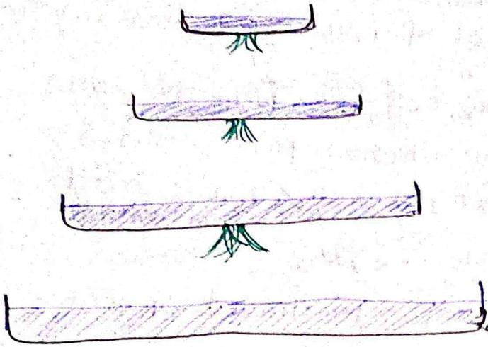
(iii) Cascade Aerator (Used for ~~less~~ treatment of water ex. ~~industry~~)
