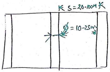
Trash  $\rightarrow$  Impurities removed by rack  $\rightarrow$  Trash rack.
