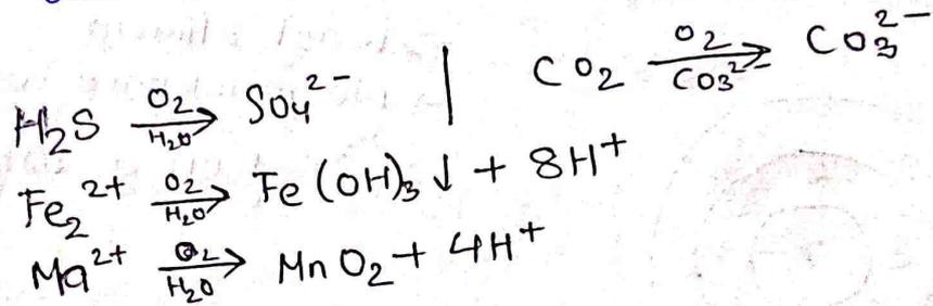
→ By aeration taste, colour, odour, pH reduces but turbidity of water increases.
