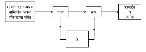
Write the name of X in the given block diagram of electric power plant.
