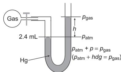
However, atmospheric pressure is measured by **barometer**. There are two types of manometers: **Closed end manometer** is normally used to measure pressure below atmospheric pressure whereas, **open end manometer** is used to measure pressure above atmospheric pressure.
