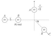
According to problem mass A moves in a perpendicular direction and let the mass B moves at angle  $\theta$  with the horizontal with velocity v.
