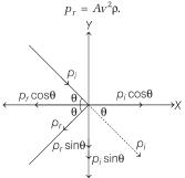
Now, making components of momentum along X and Y-axes. Change in momentum of water per second
