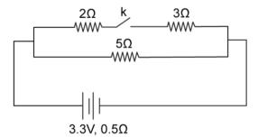
Resistance (R1) of the circuit =  $(5+0.5)\Omega = 5.5\Omega$
