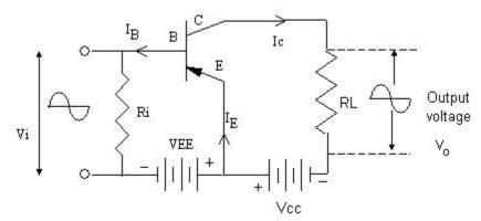
**Working principle**: In a common emitter circuit, the collector current is controlled by the base current rather than the emitter current. Since in a transistor, a large collector current corresponds to a very small base current, when the input signal is applied to the base, a very small change in the base current provides a much larger change in the collector current, and thus, extremely large current gains are possible.
