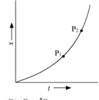
$$\overline{v} = \frac{x_2 - x_1}{t_2 - t_1} = \frac{\Delta x}{\Delta t}$$
