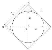
Suppose the height of transmitting antenna or receiving antenna in order to cover the entire surface of earth through communication is  $h_t$  and radius of earth is R
