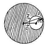
1.216 We partition the solid sphere into thin spherical layers and consider a layer of thickness dr lying at a distance r from the centre of the ball. Each spherical layer presses on the layers within it. The considered layer is attracted to the part of the sphere lying within it (the outer part does not act on the layer). Hence for the considered layer
