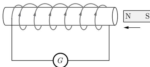
Now fix the magnet in any one position so that it is stationary with respect to the coil. We find that there is no deflection in galvanometer.
