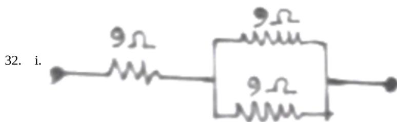
If we connected two 9 ohm resistors in parallel and other 9 ohm resistor in series as shown in figure:
