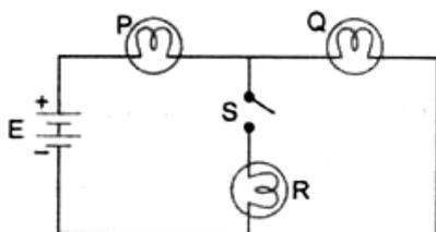
Initially the switch S is kept open and the lamp P and Q are observed to glow with same brightness. Then switch S is closed. How will the brightness of the glow of bulbs P and Q will change? Justify your answer.
