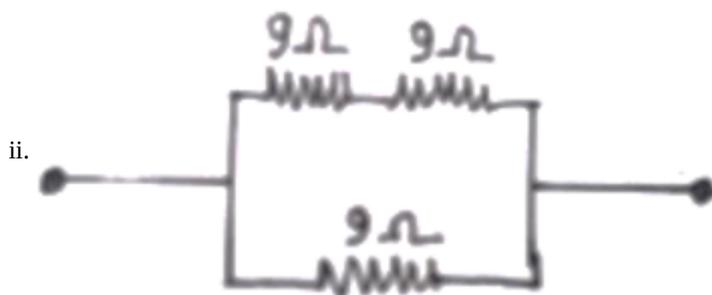
If we connected two 9 ohm resistors in series and other 9 ohm resistor in parallel as shown in figure:
