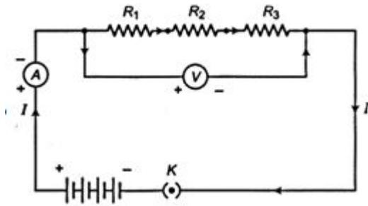
b. Given:  $R_1 = 5\Omega$ ,  $R_2 = 10\Omega$ ,  $R_3 = 15\Omega$  and  $V = 30V$
