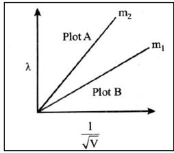
The slope of the smaller mass  $(m_2)$  is larger; therefore, plot A in the above graph is for mass  $m_2$
