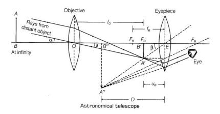
25. The ray diagram of reflecting telescope showing how ray coming from distant object are received at the eye-piece is shown in figure.
