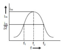
From the graph, we can see that with increase in frequency, current first increases and then decreases. At resonant frequency, current amplitude is maximum.
