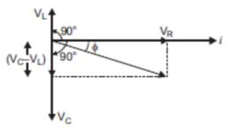
Thus,  $V_R$  and  $(V_C - V_L)$  are mutually perpendicular and the phase difference between them is  $90^{\circ}$ . As seen in the fig, we can say that, as the applied voltage across the circuit is V, the resultant of  $V_R$  and  $V_C - V_L$ ) will also be V.
