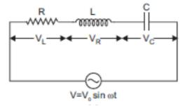
Since L, C and R are connected in series, current flowing through them is the same. The voltage across R is  $V_R$ , inductance across L is  $V_L$  and across capacitance is  $V_C$ .
