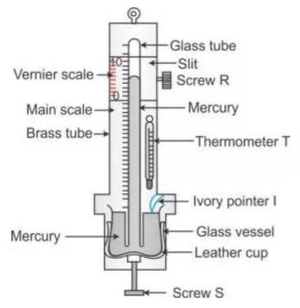
To measure the atmospheric pressure, first the leather cup is raised up or lowered down
