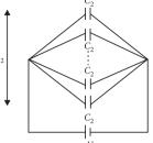
Total capacitance of the parallel combination of capacitors is  $C_p = C_2 + C_2 + \dots + upto n_2$  terms =  $n_2C_2$
