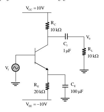
The capacitors are also assumed to be short circuited at signal frequencies. The input  $V_i$  is direct coupled. The low frequency voltage gain  $v_0/v_i$  of the amplifier is
