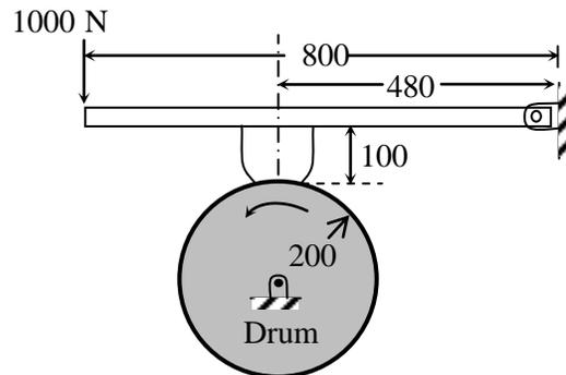
The braking torque (in N.m) for the brake shoe is \_\_\_\_\_.
