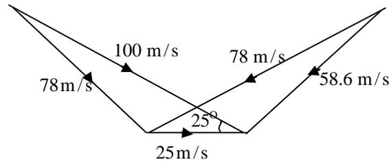
The relative velocity and the axial component of velocity remain the same between the inlet and outlet of the blades. The blade inlet and outlet velocity triangles are shown in the figure. Assuming no losses, the specific work (in J/kg) is \_\_\_\_\_.
