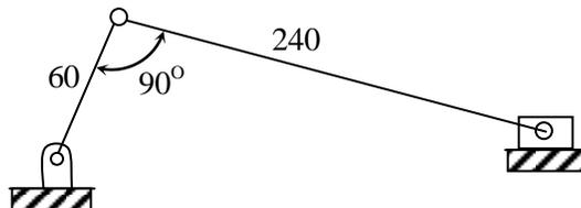
For the given configuration, the speed (in m/s) of the slider is \_\_\_\_\_.
