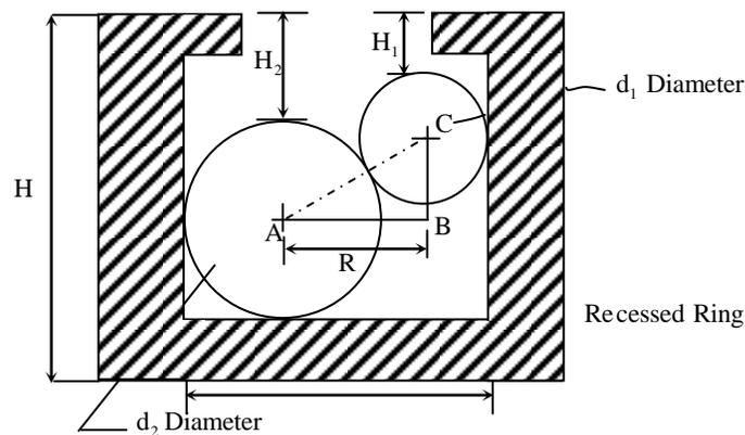
The distance  $H_2 = 35.55$  mm and  $H_1 = 20.55$  mm. The diameter ( $D$ , in mm) of the ring gauge is \_\_\_\_\_.
