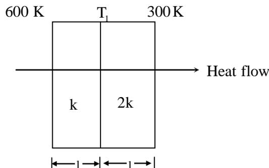
The conductivity of one section is  $k$  and that of the other is  $2k$ . The left face of the wall is at 600 K and the right face is at 300 K. The interface temperature  $T_i$  (in K) of the composite wall is \_\_\_\_\_.
