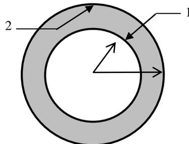
The view factor  $F_{21}$  for radiation heat transfer is
